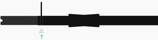
5 Holding the mounting bar horizontally with a screw facing upwards, unscrew the top screw.
